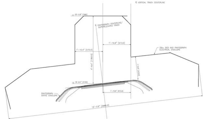
**Figure 4.10 SPACE NECESSARY FOR 25KV OVERHEAD CONTACT SYSTEM FOR CHSTP SHARED USE CORRIDORS FOR A 18'-8.4" (5700 mm) CONTACT WIRE HEIGHT IN TUNNEL OR UNDER STRUCTURE IN ALIGNMENT BETWEEN 2 SUPPORTS**
