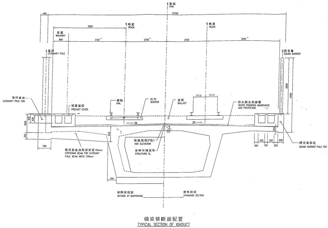
Figure 3-7: Section of Taiwan High-Speed Rail Viaduct
