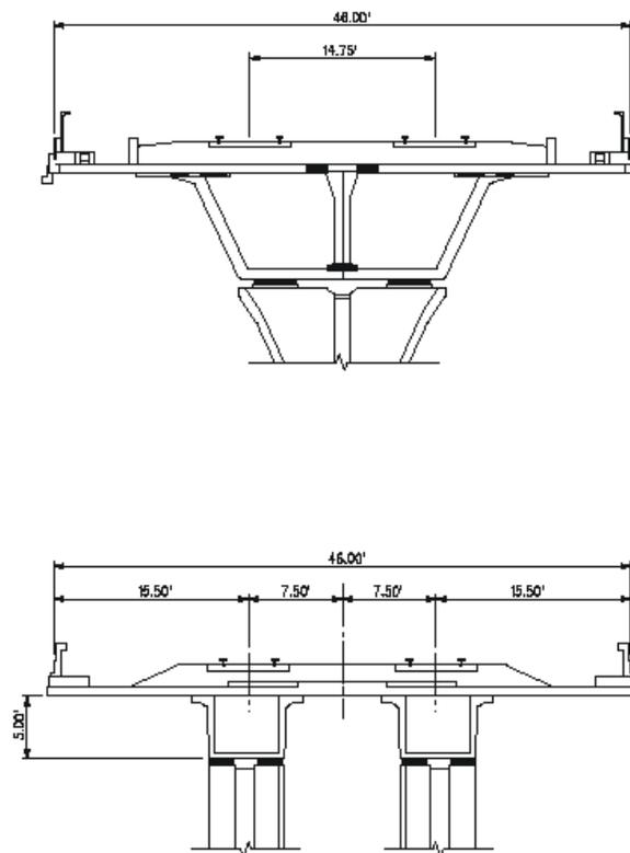
Figure 3-5: AVE Box Girder and Double Beam Cross Section
