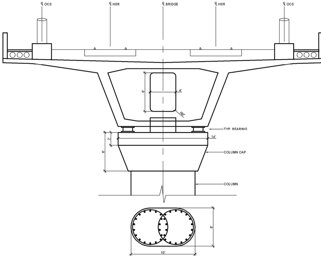
**Figure 3-11: Basic High-Speed Train Aerial Structure @ Support**
