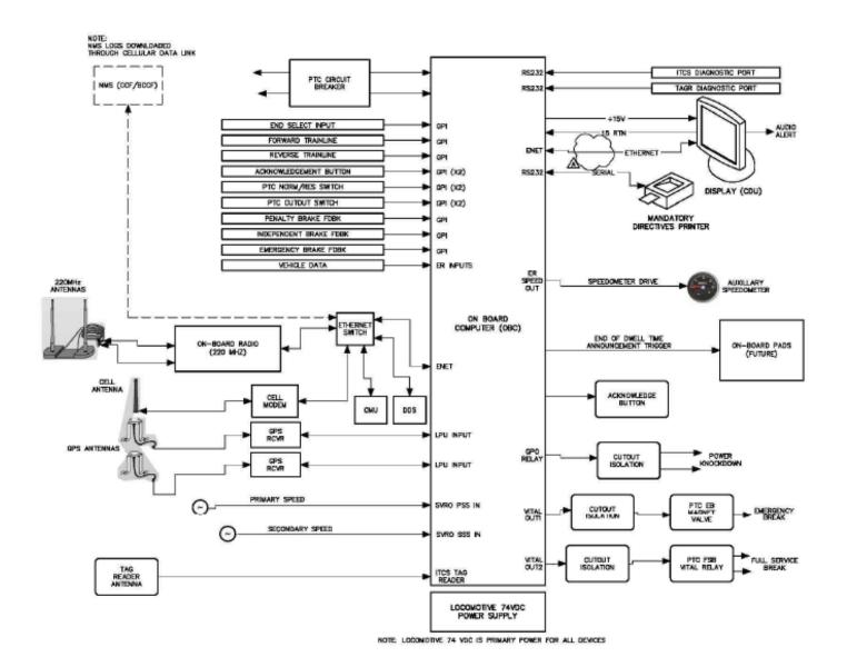
As can be seen in the above figure, the onboard PTC system requires interfaces to the vehicles, including a number of vehicle trainlines and the onboard acknowledge switch, plus multiple interfaces to the train's brake system to trigger a penalty brake application and an emergency brake application. The onboard PTC system also provides an output that may be used by the vehicle for onboard announcements.
